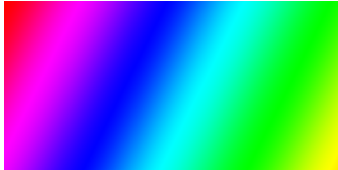
Figure 11: Rainbow pattern with spatially varying wavelength illumination used in single-shot structured light techniques
